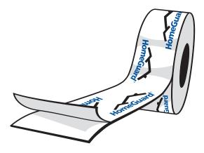
HomeGuard<sup>®</sup> Titan<sup>®</sup> Butyl Flashing is a high tack, high performance self-adhered window and door flashing tape designed with a wide application temperature range from 20°F to extreme heat of 160°F without requiring primer or mechanical fasteners. Available in 4", 6", 9" and 12" x 75' rolls.
