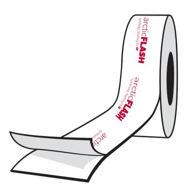
Arctic-Flash® is a high tack, high performance self-adhered window and door flashing tape designed with a wide application temperature range from 0°F to extreme heat without requiring primer or mechanical fasteners. Available in 4″, 6″ and 9″ x75′ rolls.
