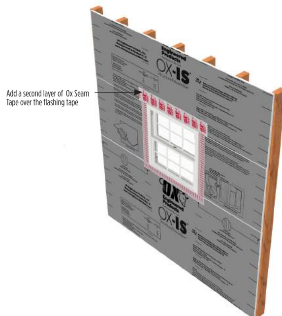
Detail I - Completed installation
