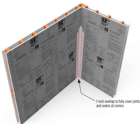
Detail F - Interior corner flashing tape
