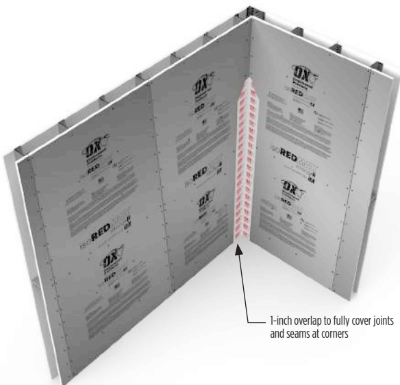
Detail F - Corner flashing tape
