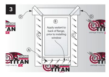
To integrate windows and doors properly into housewrap, follow these steps; **A)** Install the window flashing on the sill flush with the rough opening. **B)** Apply 3/8" bead of **HomeGuard** \* **Polymer Sealant** to the back side of the window flange and secure the window in place. **C)** After the window is set, apply flashing to both jambs. **D)** Install the head flashing and re-integrate the head flap with **HomeGuard** \***Seam Tape**
