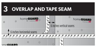
At vertical and horizontal seams, apply a minimum of 6" vertical overlap. When going around corners, make sure housewrap is pulled tightly and properly fastened. Any succeeding course should be placed horizontally over the lower course in a weather-board fashion with a minimum horizontal overlap of 6". Use **HomeGuard** \* **Seam Tape** to seal all seams.
