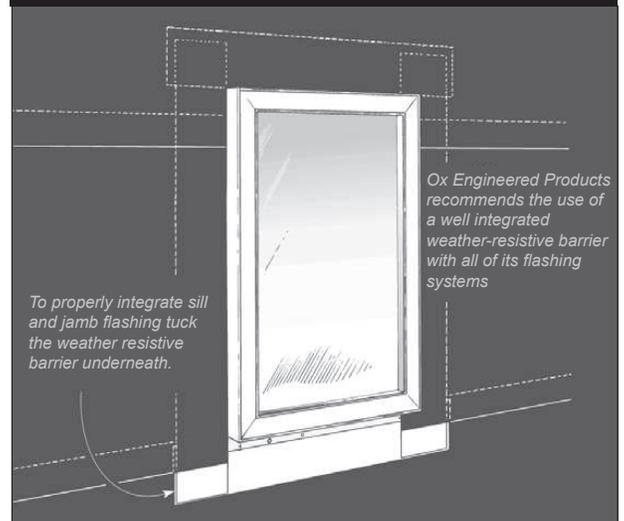
This recommendation refers to the most common types of windows used (surface mounted). For other types of frames, special attention should be paid to the window manufacturer's instructions.
