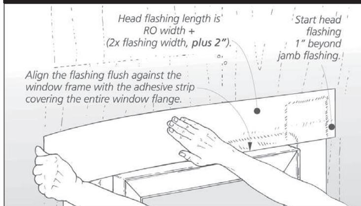
Wipe the head flange, jamb flashing and sheathing with a clean rag. Cut the head flashing to twice the width of the rough opening + 2x the width of the flashing plus 2". Install the head flashing by pressing firmly in place in one direction to prevent voids.
