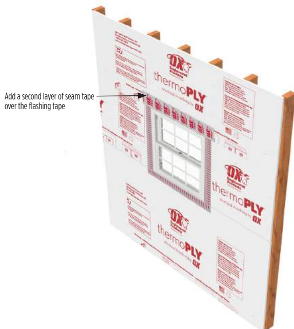
Detail K- Completed installation
