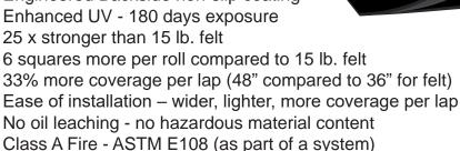
**ToughSkin 15** 1,000 ft<sup>2</sup> (10 Squares) Roll Size 48" x 250' **Roll Dimensions** Weight per Roll 19 lbs / Roll Rolls per Pallet 64 **UV** Exposure Limit 6 months (MAXIMUM) Tensile Strength ASTM D1970 MD=85 | CD=54 Tear Strength ASTM D5733 MD=35 | CD=36
