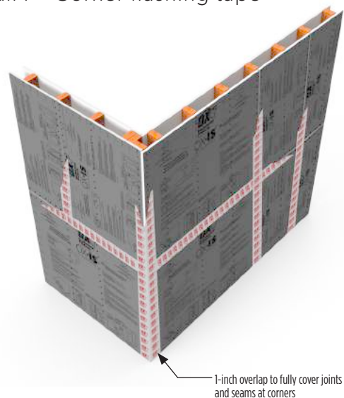
Detail F - Corner flashing tape
