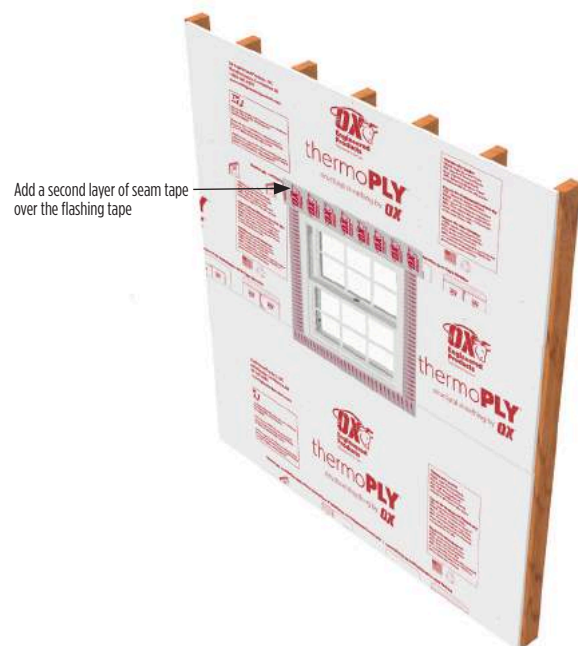
Detail J - Completed installation
