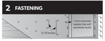
HomeGuard recommends using a minimum 1" plastic cap fasteners (minimum 15/16" crown staples that penetrate the studs are acceptable) to attach housewrap so that is taut and flat. The proper spacing for these fasteners is 12" to 18" on center. Guide marks have been printed every 8" to help locate studs.
