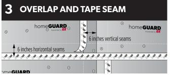
At vertical and horizontal seams, apply a minimum of 6" vertical overlap. When going around corners, make sure housewrap is pulled tightly and properly fastened. Any succeeding course should be placed horizontally over the lower course in a weather-board fashion with a minimum horizontal overlap of 6". Use **HomeGuard**<sup>®</sup> **Seam Tape** to seal all seams.
