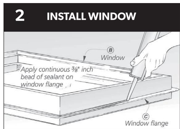
Before installing the window, apply a continuous 3/8" bead of HomeGuard Polymer Sealant to the back side (interior) of the mounting flange. Install the window according to the window manufacturer's instructions.
