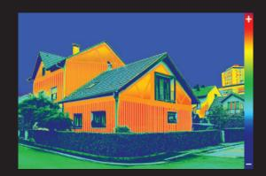
Without continuous insulation, heat loss through framing (thermal bridging) is significant.
