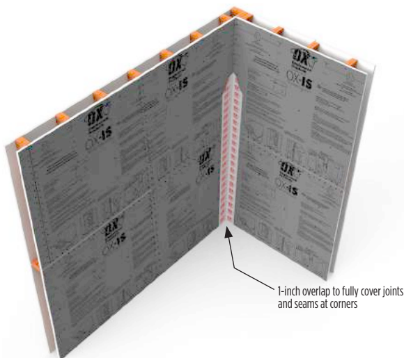
Detail G - Interior corner flashing tape
