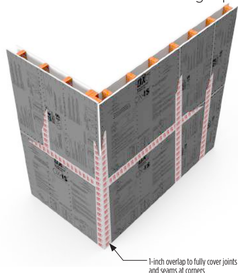
Detail H - Exterior corner flashing tape
