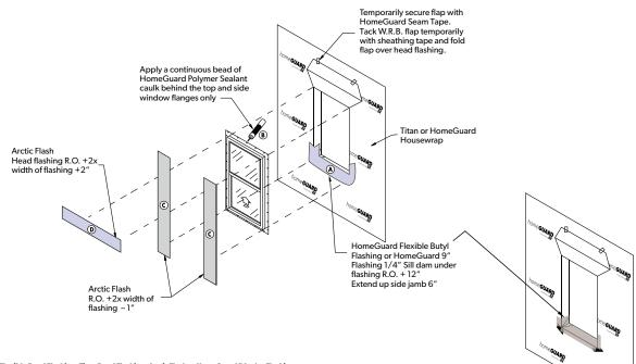
A. HomeGuard Flexible Butyl Flashing, Titan Butyl Flashing, Arctic Flash or HomeGuard RA-plus Flashing
