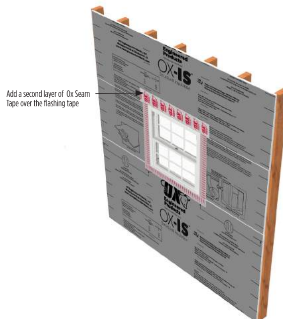
Detail J - Completed installation
