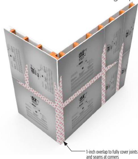
Detail H - Exterior corner flashing tape
