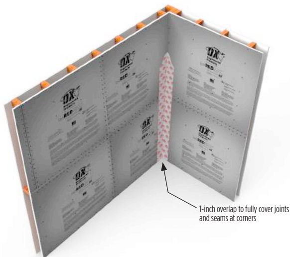
Detail G - Interior corner flashing tape
