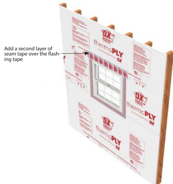
Detail L- Completed installation
