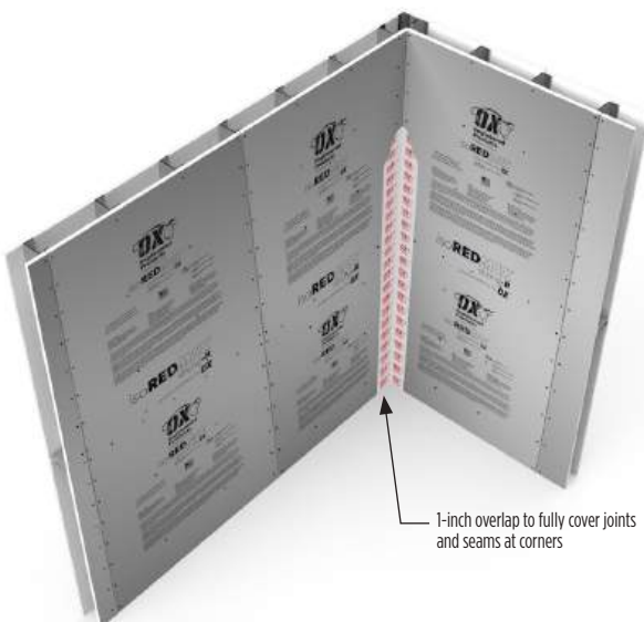
Detail F - Corner flashing tape
