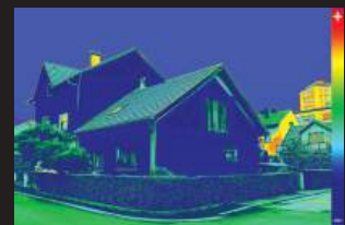
THERMAL IMAGE OF THE SAME STRUCTURE BUILT WITH 1/2" (R-3) OF CONTINUOUS INSULATION
