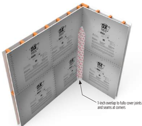
Detail G - Interior corner flashing tape
