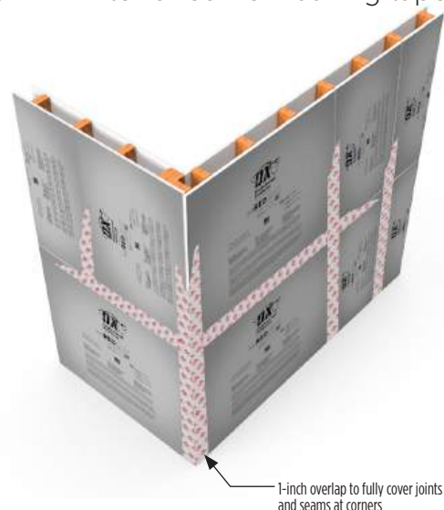
Detail H - Exterior corner flashing tape
