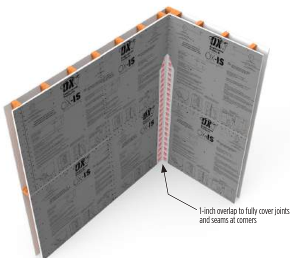
Detail G - Interior corner flashing tape
