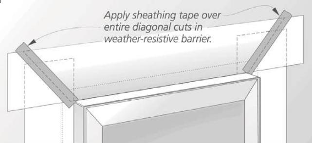
Finally, allow the flap of the weather-resistive barrier at the head to lay flat over the head flashing. Apply a new piece of sheathing tape over the entire diagonal cut made in the weather-resistive barrier and press firmly in place.
