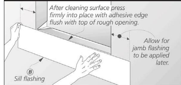
Cut the sill flashing to the width of the rough opening plus twice the flashing width. Wipe the surface of the weather-resistant barrier with a clean rag to ensure proper adhesion. Remove the release paper and press the sill flashing in place so that the edge of the flashing's adhesive is level with the top edge of the rough opening.
