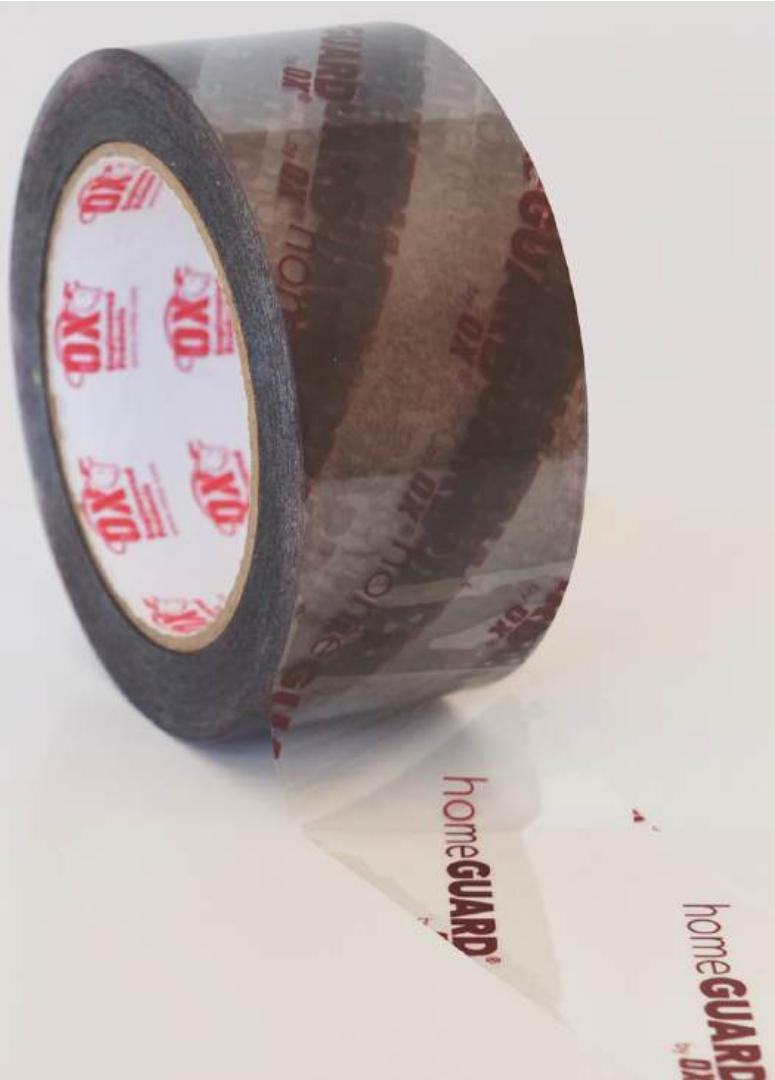
HomeGuard® SeamTape® is a polypropylene sheathing tape coated with an aggressive acrylic pressure sensitive adhesive (PSA) designed for use as a closure system and vapor seal on all interior and exterior sheathing materials. HomeGuard® SeamTape® is the highest performing, highest value product on the market today. Available in white, 1 7/8" x 165', and 2 7/8" x 165'
