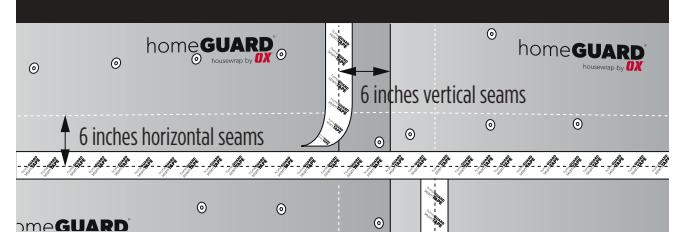
At vertical and horizontal seams, apply a minimum of 6" vertical overlap. When going around corners, make sure housewrap is pulled tightly and properly fastened. Any succeeding course should be placed horizontally over the lower course in a weather-board fashion with a minimum horizontal overlap of 6". Use **HomeGuard® Seam Tape** to seal all seams.
