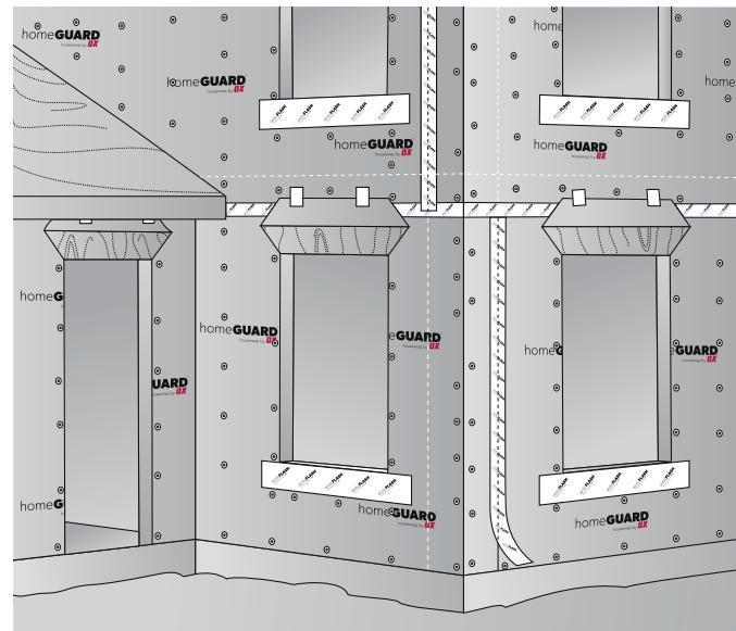
\* Asphalt flashing products should not be used with Titan Drainage Wrap
