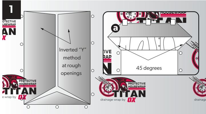
At the rough opening, cut housewrap in an inverted "Y" fashion, and then fasten with the methods described in **Step 2**. To allow for head flashing integration, make a 45° cut in housewrap as shown above in detail **a**. Ensure that any protrusions in the wall assembly including windows, doors, vents, hose bibs and electrical boxes are flashed and integrated properly into housewrap.
