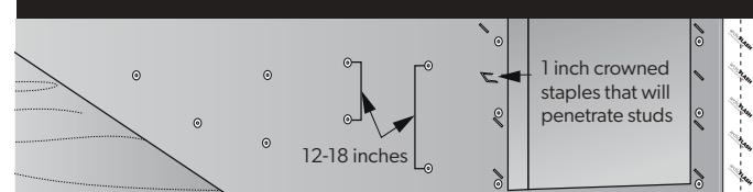
HomeGuard® recommends using a minimum of 1" plastic cap fasteners (using fasteners without a plastic cap is acceptable if they are a minimum of 15/16" crown staples) to attach housewrap so that it is taut and flat. The proper spacing for these fasteners is 12" to 18" on center. Guide marks have been printed every 8" to help locate studs.
