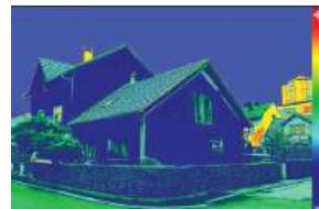
**Thermal image of the same structure built with 1/2" (R-3) of continuous insulated sheathing.**
