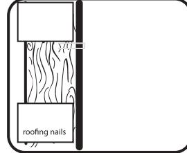
Use 16 gauge 1" crown, 1 1/4" length staple OR 11ga/ 1 1/4" length roofing nail. Staple crown should be flush. DO NOT countersink Staples must run parallel with wood grain of framing studs at sheathing seams.
