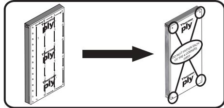
Install vertically or horizontally. Fastener pattern for structural: 3" / 3" o.c.; up to 6" / 12" o.c. Refer to DrJ Technical Evaluation Report for complete specifications. Start at one edge of the panel and move sequentially across to opposite edge.
