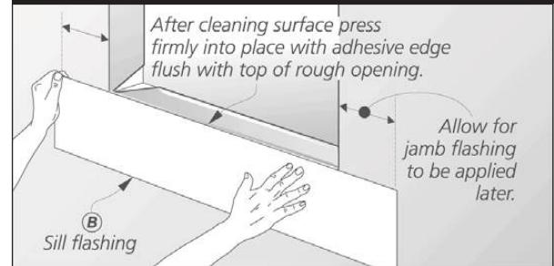
Cut the sill flashing to the width of the rough opening plus twice the flashing width. Wipe the surface of the weather-resistive barrier with a clean rag to ensure proper adhesion. Remove the release paper and press the sill flashing in place so that the edge of the flashing's adhesive is level with the top edge of the rough opening.
