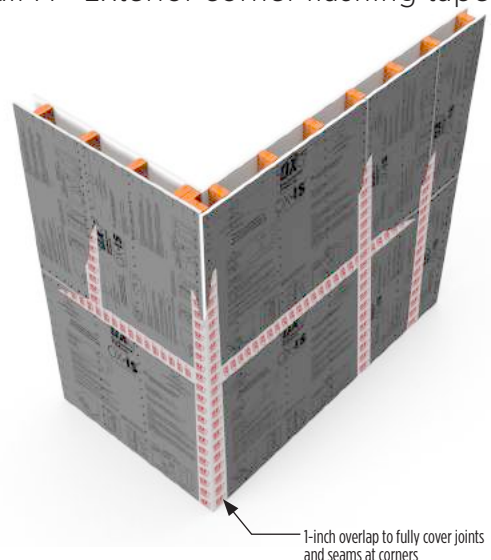
Detail H - Exterior corner flashing tape
