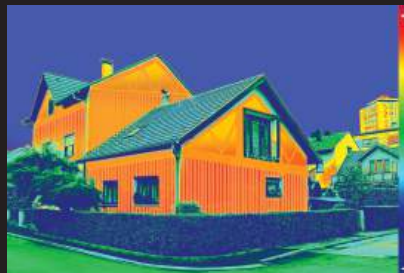
THERMAL IMAGE OF A STRUCTURE BUILT WITHOUT INSULATED SHEATHING
